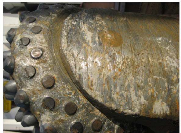
Figure 8. Worn roller cone bit.
