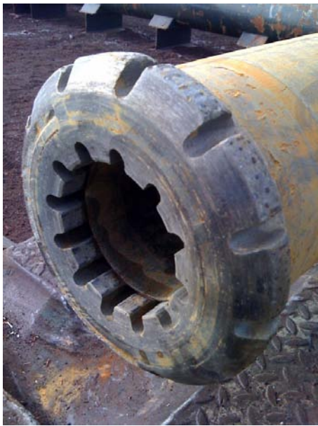
Figure 10. The Core bit after the coring attempt.
