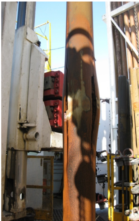
Figure 11. The 8" DC after the explosion.
